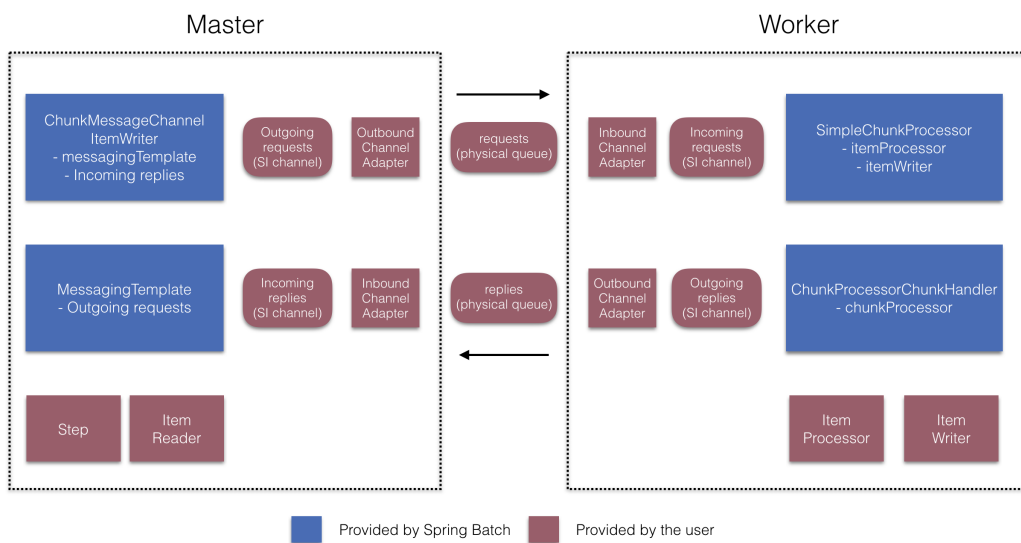
Figure 31. Remote Chunking Configuration
